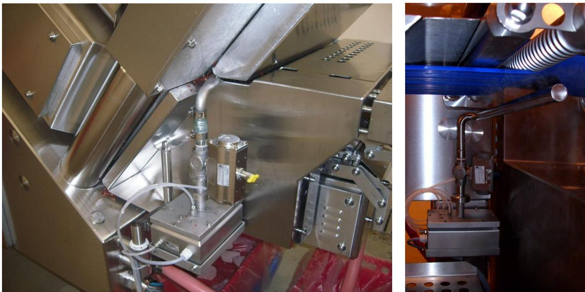
Picture 1 und 2: Fogging units at Slicier-Knife and a conveyor belt
