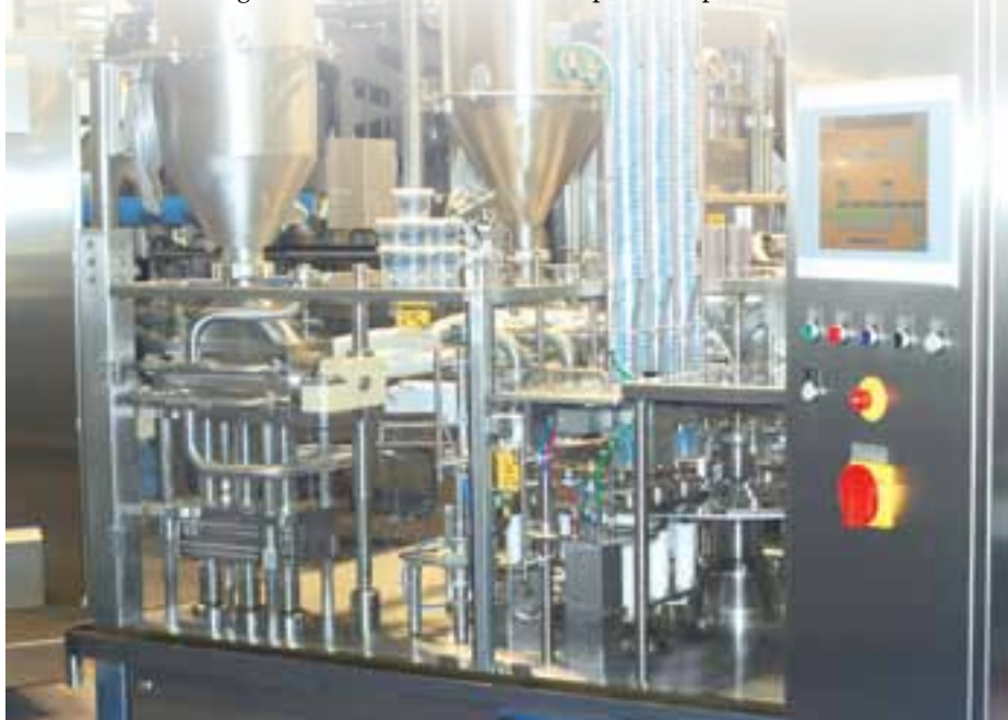
Servo motor driven cup filling and closing machine with integrated sterilisation system
